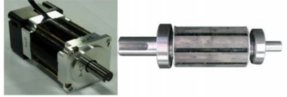
Fig. 4. The experiment motor and the surface mounted magnet rotor
